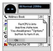
After the first start press the "Option" button on the lower panel and select checkbox "Enable FastCPU" to activate the program.
